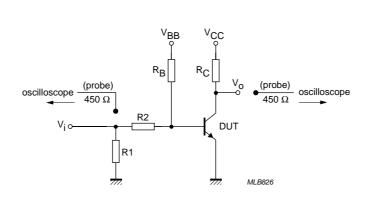
$V_i$  = 5 V; T = 500  $\mu s;$   $t_p$  = 10  $\mu s;$   $t_r$  =  $t_f \leq 3$  ns.
