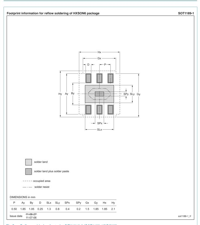
Fig 5. Reflow soldering footprint DFN1616-6 (SOT1189-1/XSON6)
