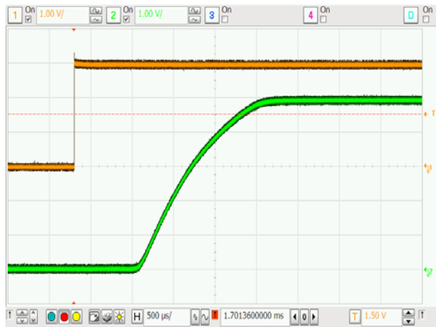
Figure 19. Turn-on Response (V CC = 3.3 V, V IN = 5.0 V, R L = 10 Ω, C L = 0.1 μF)
