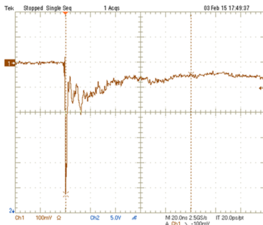
Figure 2. IEC61000-4-2 -8kV Contact ESD Clamping Voltage
