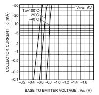
Fig.1 Grounded emitter propagation characteristics
