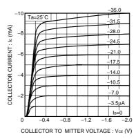
Fig.2 Grounded emitter output characteristics (I)
