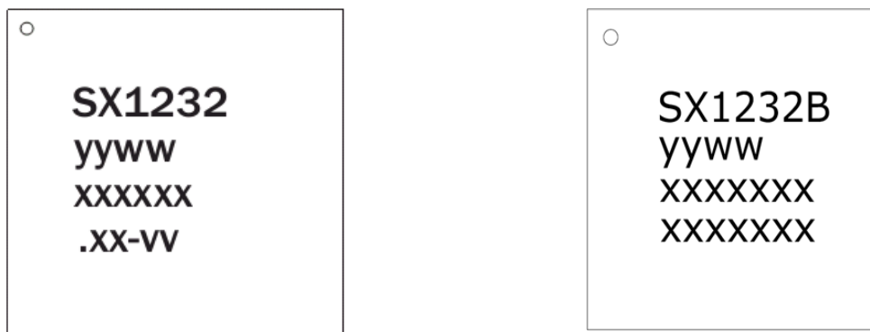
Figure 3. Marking Diagram SX1232 & SX1232B
