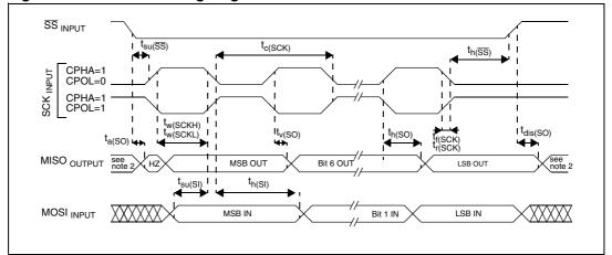
Figure 82. SPI slave timing diagram with CPHA =  $1^{(1)}$
