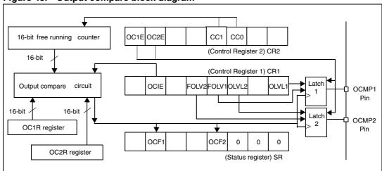
Figure 43. Output compare block diagram
