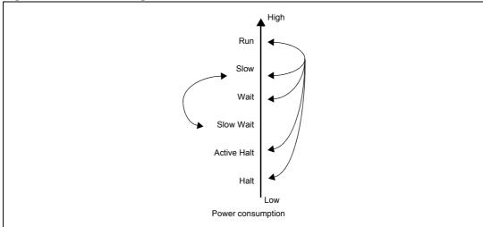
Figure 23. Power saving mode transitions
