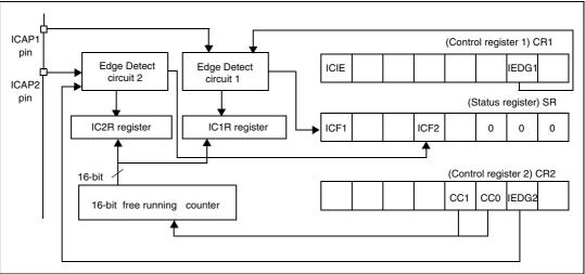
Figure 41. Input capture block diagram
