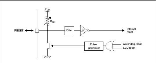
The RESET pin is an asynchronous signal which plays a major role in EMS performance. In a noisy environment, it is recommended to follow the guidelines mentioned in the electrical characteristics section.
