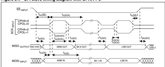
Figure 81. SPI slave timing diagram with CPHA =  $0^{(1)}$
