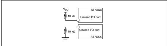
1. I/O can be left unconnected if it is configured as output (0 or 1) by the software. This has the advantage of greater EMC robustness and lower cost.
