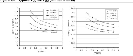
Figure 75. Typical V<sub>OL</sub> vs. V<sub>DD</sub> (standard ports)
