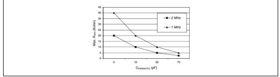
C<sub>PARASITIC</sub> represents the capacitance of the PCB (dependent on soldering and PCB layout quality) plus the pad capacitance (3 pF). A high C<sub>PARASITIC</sub> value will downgrade conversion accuracy. To remedy this, f<sub>ADC</sub> should be reduced.
