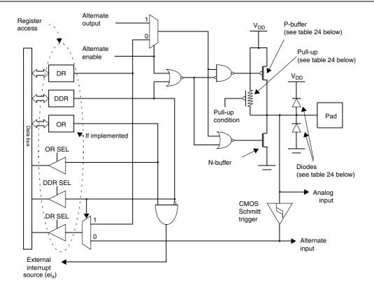
Figure 30. I/O port general block diagram
