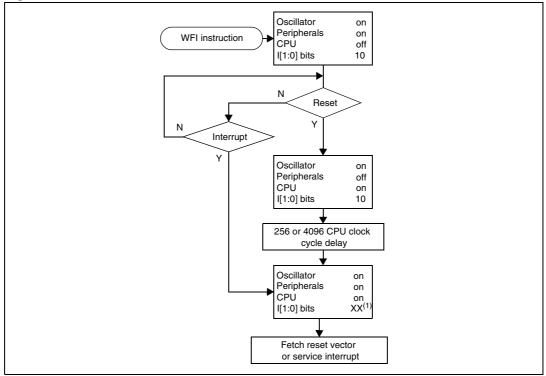
Before servicing an interrupt, the CC register is pushed on the stack. The I[1:0] bits of the CC register are set to the current software priority level of the interrupt routine and recovered when the CC register is popped.
