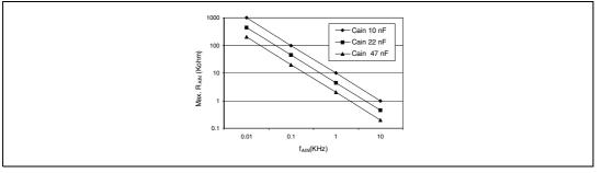
1. This graph shows that, depending on the input signal variation ( $f_{AIN}$ ),  $C_{AIN}$  can be increased for stabilization time and decreased to allow the use of a larger serial resistor ( $R_{AIN}$ ).
