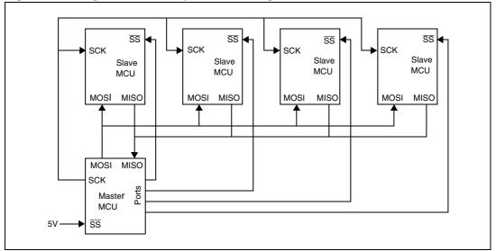
Figure 56. Single master/multiple slave configuration
