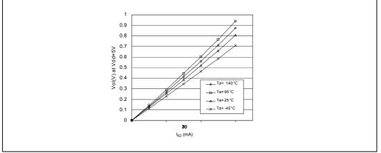
Figure 74. Typical  $V_{OH}$  at  $V_{DD}$  = 5 V
