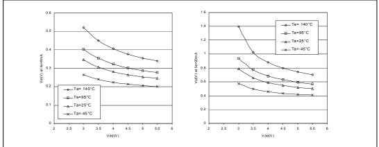
Figure 77. Typical V<sub>OH</sub> vs. V<sub>DD</sub>
