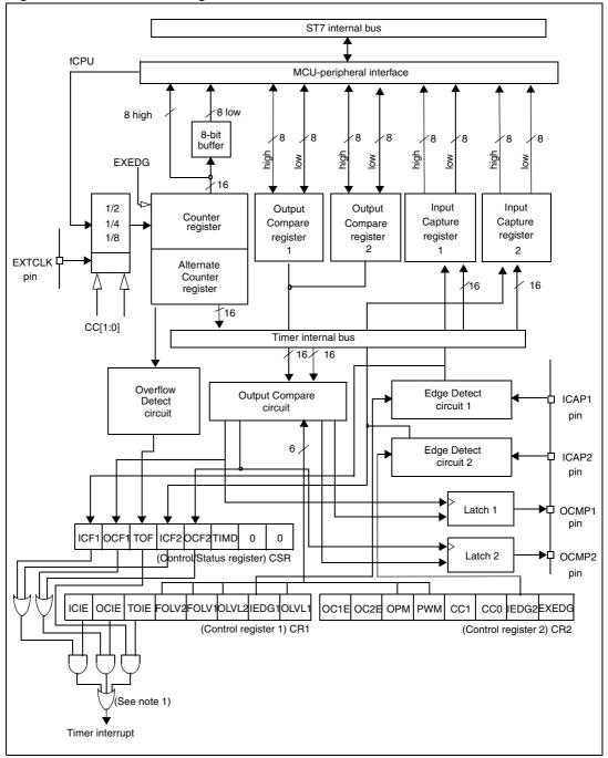
Figure 36. Timer block diagram
