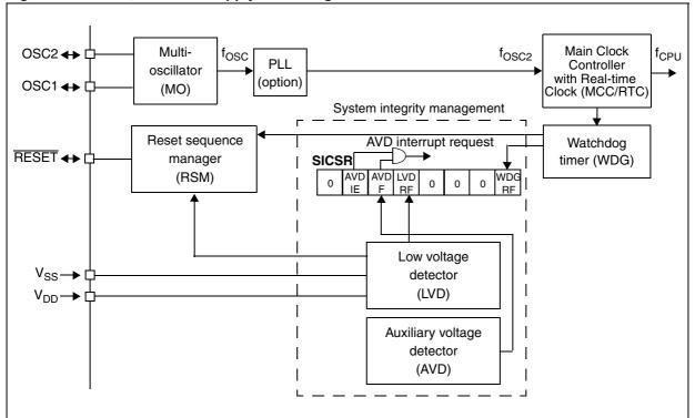
Figure 12. Clock, reset and supply block diagram
