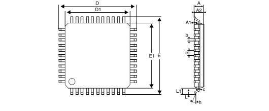
Table 114. 44-pin low profile quad flat package mechanical data
