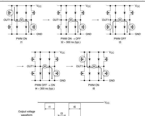
Note: Be sure to set the pin PWM to High when the PWM control function is not used.
