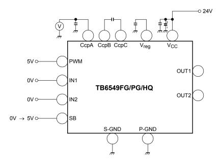
•  $tong: SB = 0 V \rightarrow 5 V$ . Measure the time taken to boost the CcpA voltage up to about 29 V (24 V + 5 V).
