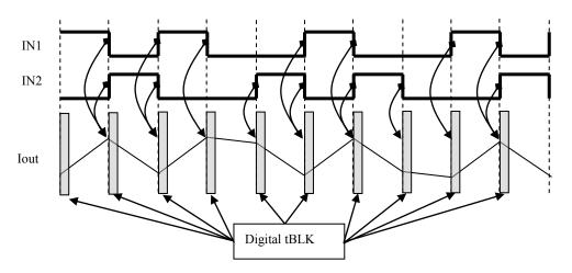
The Digital tBLK is inserted at the beginning of each charge period of the constant current chopping, and also when either the INA1/A2/B1/B2 is switched.
