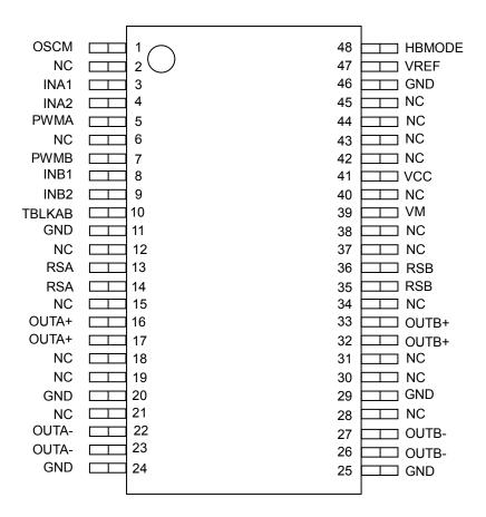
Note: Please connect the exposed pad to the PCB ground pattern when using the HTSSOP package.
