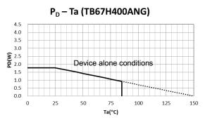
This value is dependent on a substrate pattern and mounting conditions. Moreover, when ambient air temperature is high, permissible power consumption becomes small.
