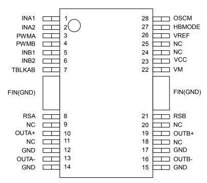
Note: Please connect the FIN(GND) to the PCB ground pattern when using the HSOP package.
