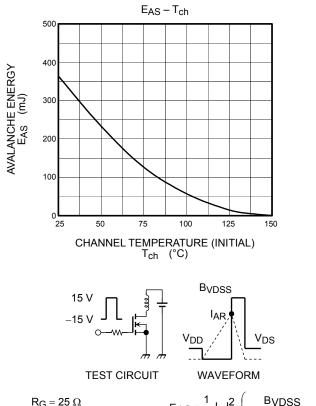
$$E_{AS} = \frac{1}{2} \cdot L \cdot I^2 \cdot \left( \frac{B_{VDSS}}{B_{VDSS} - V_{DD}} \right)$$
