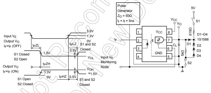
${\sf C}_{\sf L}$  is approximately 15pF which includes probe and stray wiring capacitance.
