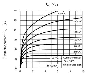
Collector-emitter voltage  $V_{CE}$  (V)
